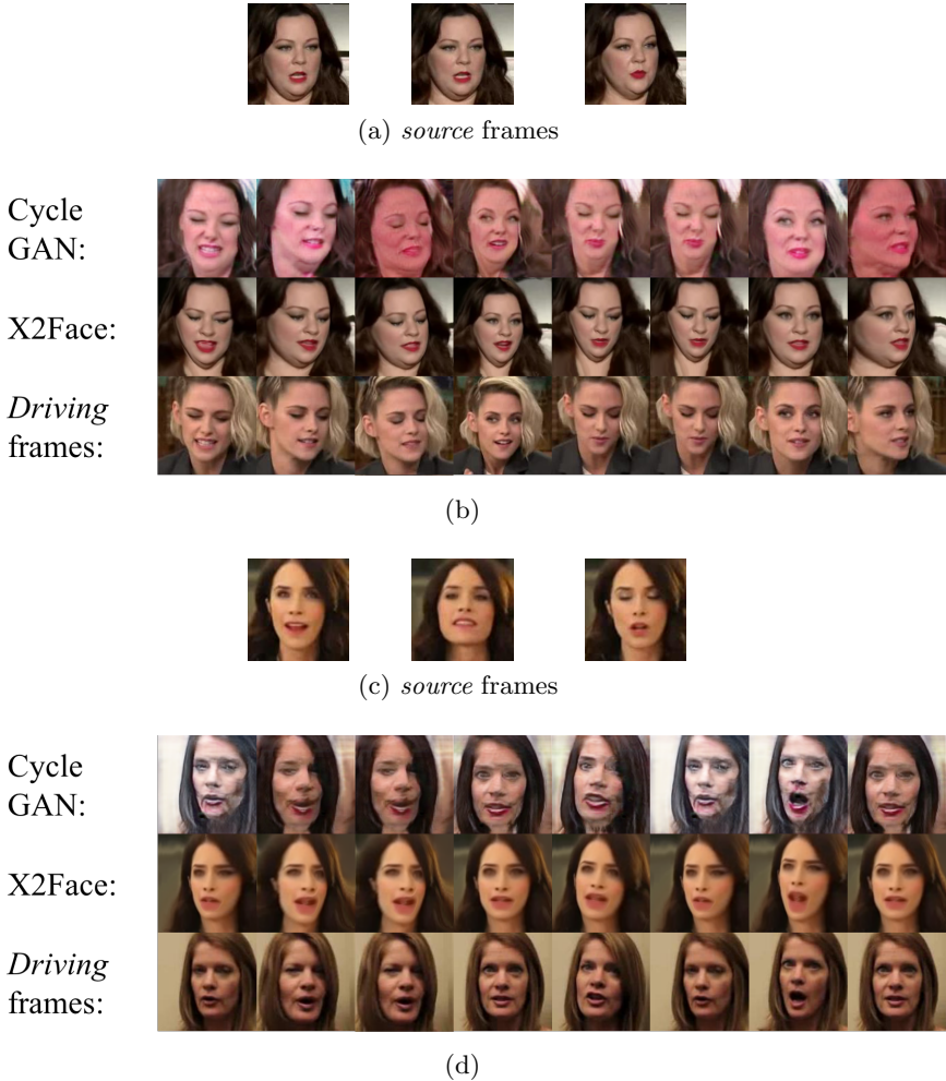
Fig.12: More qualitative results comparing X2Face to CycleGAN. Note how X2Face preserves the hair/background setting from the source frames, resulting in temporal coherence across the generated frames.
